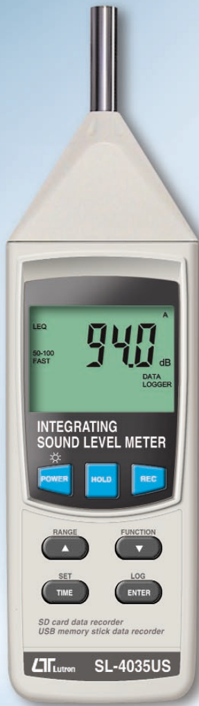
SD card/USB memory stick data recorder INTEGRATING SOUND LEVEL METER, class 2 Model : SL-4035US
