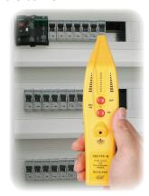
The Circuit breaker that supplies the Transmitter circuitry is the one, that (when pointed out by the tip) has the most LEDs lit on the bar-graph and the fastest buzz.
