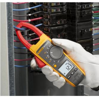
Measuring current with a clamp meter.
