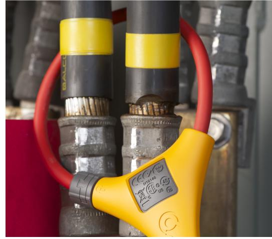
Use a flexible current probe for situations like this, where large conductors make it difficult to use the clamp meter jaws.
